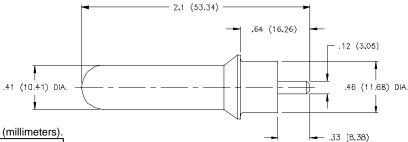
Drawing dimensions in inches and (millimeters).
